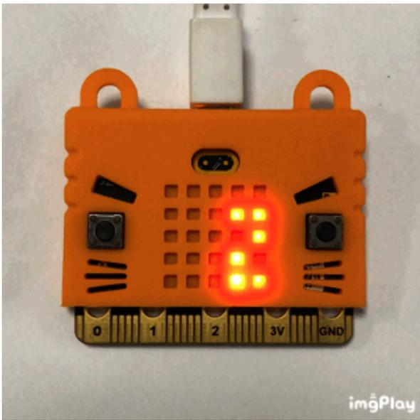
Formally connect to Bluetooth. If you can't find Bluetooth, please refresh it and select the MICRObit you want to connect. (You can see that the ID shown by the red line is the same as the one displayed by the above Microbit, so the Microbit corresponds.)
