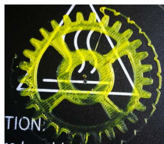
Gap is too narrow between nozzle and Hotbed, reduce the Z-height by 0.1~0.3mm
