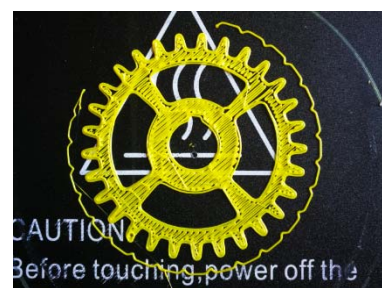
Gap is too large between nozzle and Hotbed, increase the Z-height by 0.1~0.3mm
