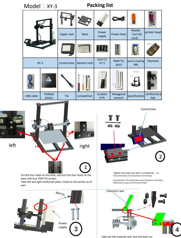
Run 2PCS M4\*25 screws through the front z-axis profile and lock the power on the back of the profile.
