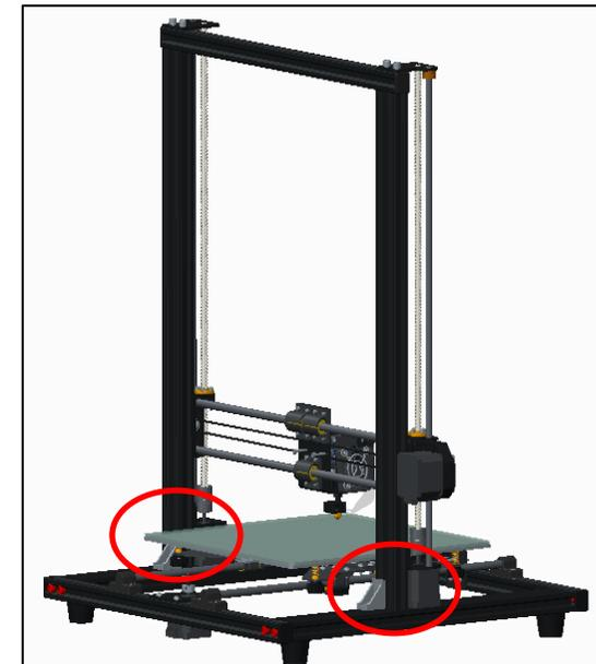
Attention: Put the vertical frame on the chassis, align it with the holes on the aluminum profile of the chassis, and fix to on the chassis with 4 M5 \* 20 screws.
