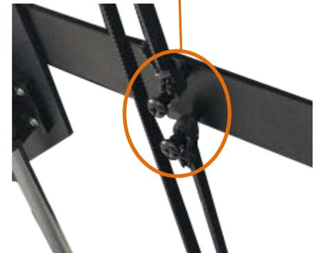
Note: The belt is cut to a proper length and fixed on the two M4 \* 14 crews in step 6, Please tighten the belt and press it to see if it is loose.
