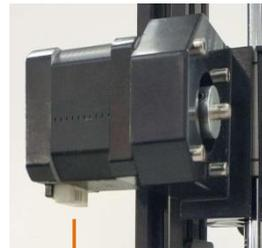
The motor connection port is facing down, as shown in the figure
