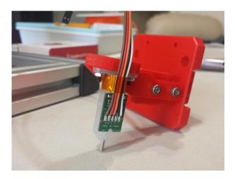
The mount needs to be adjustable so that the distance between the bottom of the sensor (not the pin) needs to be 8.3mm above the tip of the nozzle. The sensor should also be at least 15mm away from the hot bits.
