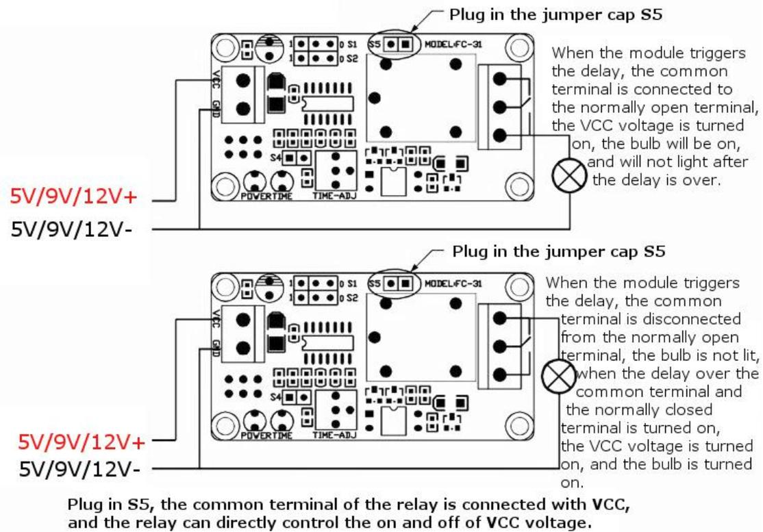
When S5 is plugged in VCC and the common terminal of the relay will be connected. If the relay controls the AC, it cannot be plugged in, otherwise the high voltage will flow back into the module, and the module will burn out.
