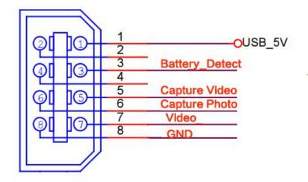
**Battery\_Detect:** Detect voltage of the battery.Note: GND need to connect. **Capture video/photo:** Trigger to capture, active low(>250ms) **Video:** video out.
