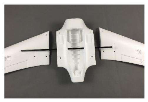
2. **Locate Right and Left wings** and slide each side over the spar until they reach the center. *Aileron servos should be on top.*
