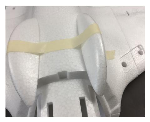
6. **Locate rudders, screws and secure into place**. It is not necessary to glue the rudders into place.
