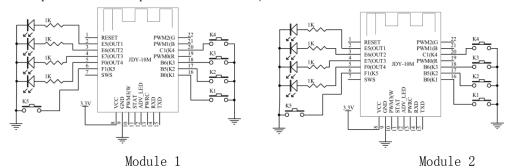
Description: the key of module 1 can control the LED light of module 2, and the key of module 2 can also control the LED light application of module 1. Note that the type of the two is AT+CLSSAO, of course, the short address of the key needs the user's own configuration. The above module 1 and module 2 are only an example, not only support two modules to control each other, but can also support dozens of module control.
