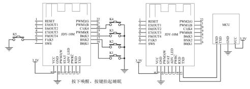
Note: the low power consumption telecontroller must pre configure the module to AT+CLSSCO type, so that when the button is not pressed, the current will be several uA. When the button is pressed, the transmit key value is waken up.
