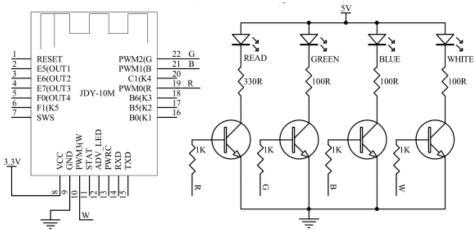
Note: LED light application, we must pre configure the module to AT+CLSSB1 type, supporting hundreds of LED lights mesh networks control.
