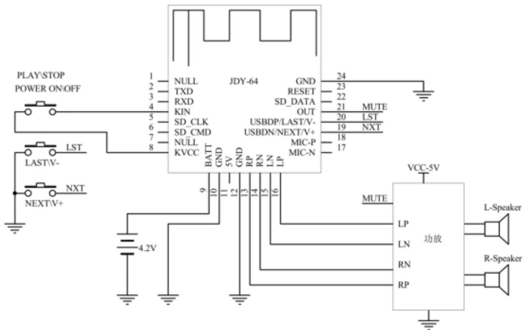
Bluetooth stereo speaker schematic diagram
