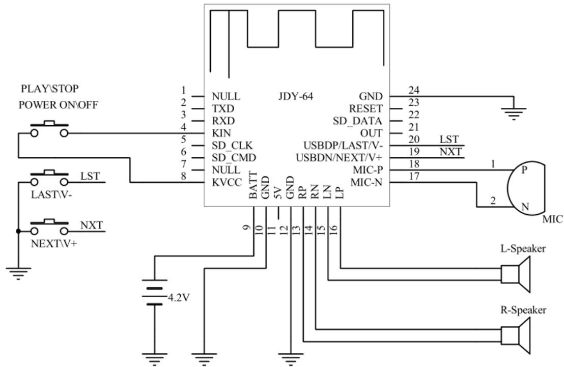
Schematic diagram of two-channel Bluetooth headset
