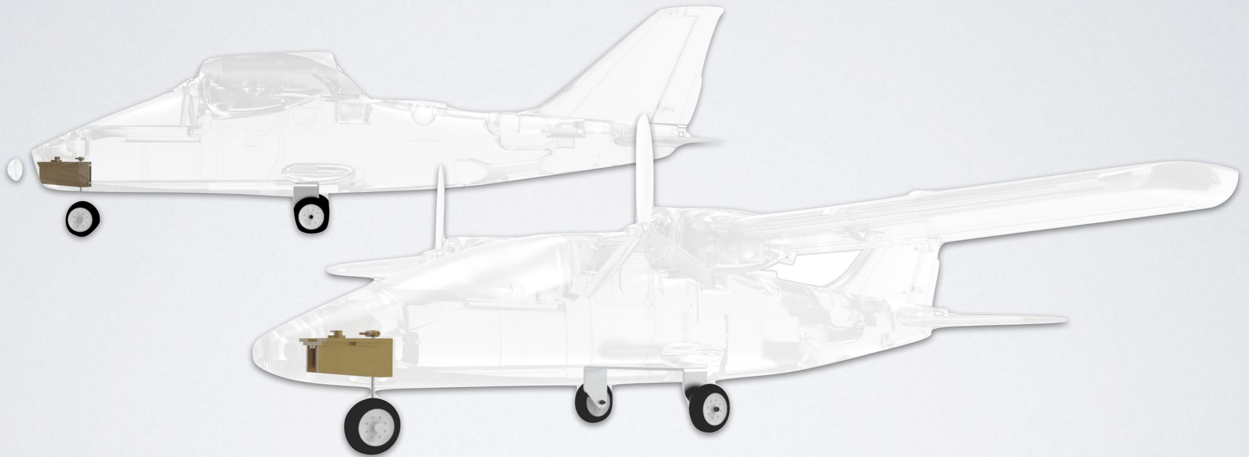
Modular landing gear: Front and rear landing gear set.
