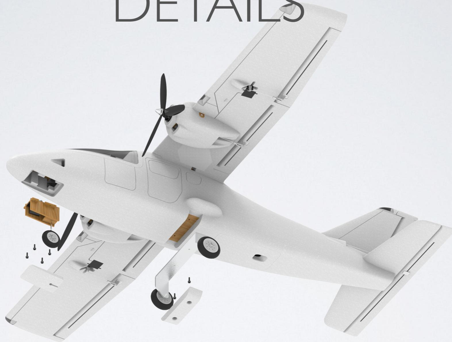
We have successfully tested Binary taking off with 3kg AUW (all-up weight). For those heavier setups, you may want to take off from a runway. A high quality aluminum rear landing gear and light weight yet strong nose gear (3mm wire) will let you do that without sweating.
