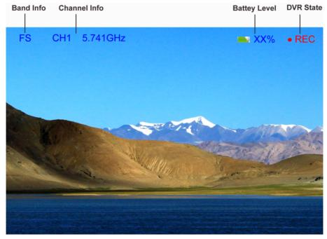
Band: The abbreviation for the radio frequency band that the headset is currently on.
