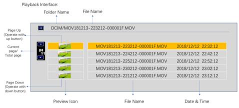
Once the desired file is selected, the screen will go into a video playback screen. The Playback OSD will indicate the playback status (playing, paused, fast forward, or fast rewind). It will also show the current file number, the name of the movie file, and the date / timestamp of the file.
