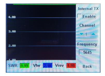
Realtime mode allows to check SWR using external(no longer support) or internal transmitter (switchable with Enable check box).
