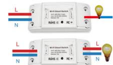
\*Note: The WiFi Switch must be powered up by N and L wires.
