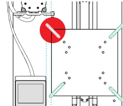
Make sure the fixtures don't impede the movement of the linear modules.
