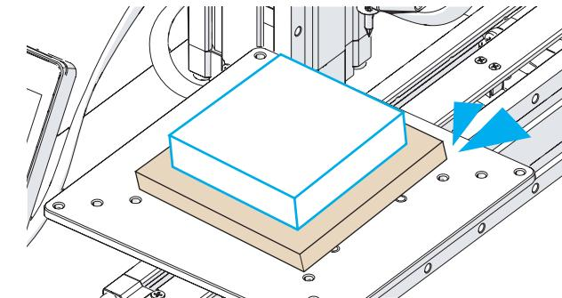
If you need to cut through the material, a spoilboard Must be put under the material to avoid damaging the CNC bit and the Engraving & Carving Platform.
