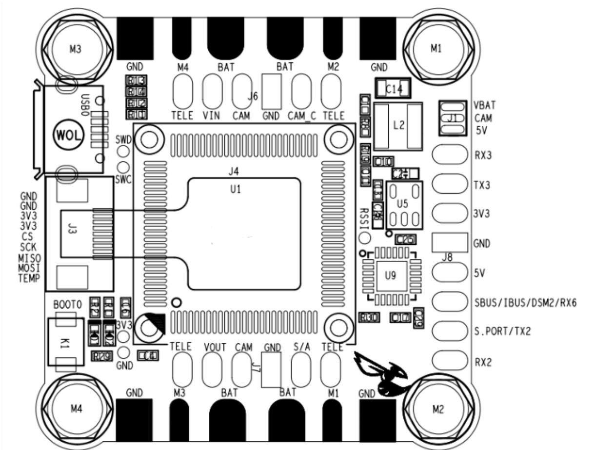
To get started on the build process with your new Betaflight F7 please take a moment to familiarize yourself with the wiring of the flight controller. Click on the picture above to direct yourself to an expandable view of the flight controller.
