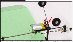
电池粘到底板, 电池插头插入接收机, 即可进行对频调试, Paste the battery to the bottom plate, and get power from the receiver for on-frequency debugging
