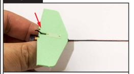
把尾翼穿入C机身尾部滑橇,注意加强片朝向。 Insert the tail into the tail of the C fuselage, pay attention to the orientation of the reinforcement.
