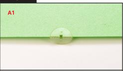
从B上撕下上图加强片,对齐机翼槽口粘贴加强片。 Remove the above reinforcement sheet from the B,and align the wing slot with the reinforcement sheet.
