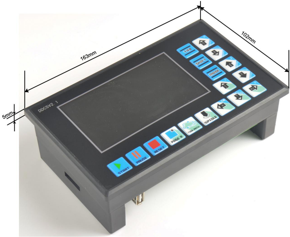
Picture1-1 DDCSV2.1Front external view and dimension figure
