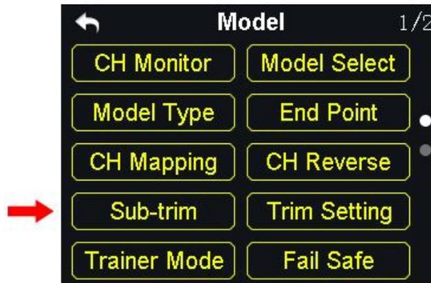
Sub-trim function helps users set channel's middle position and do trim adjustment to aircraft's flight attitude.
