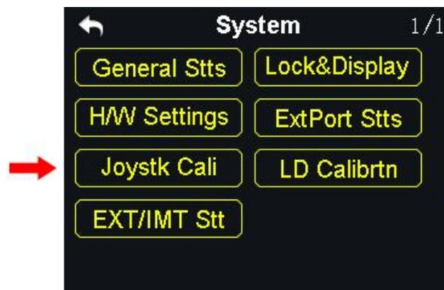
Joystick calibrating function help users calibrate joysticks' middle position.
