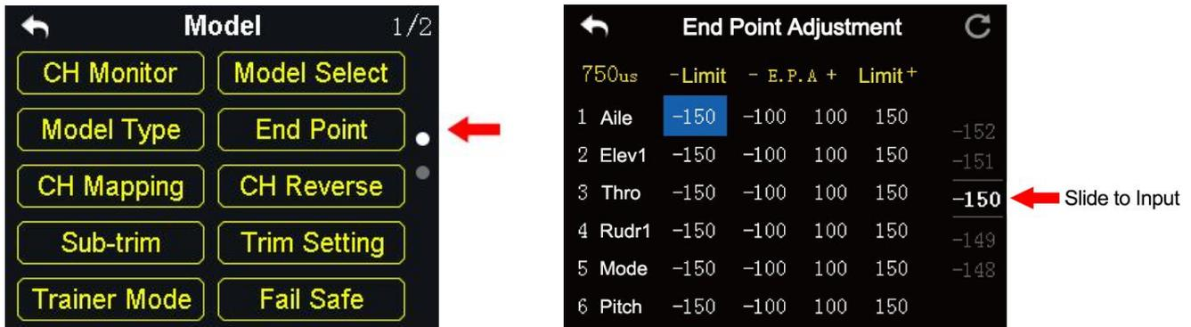
End point function helps users adjust channel value and the maximum / minimum limit on both ends.
