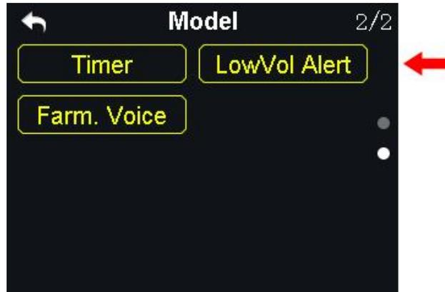
XT32 transmitter’s power telemetry function helps users set voltage alert. When aircraft’s power voltage is lower than a safe level, users receive voice and vibration alert from transmitter.
