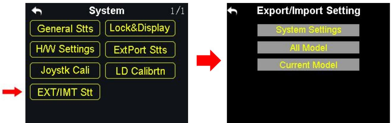
Export setting function helps user export XT32 transmitter’s system settings, model settings data to SD card, sharing the settings to other XT32 transmitters.
