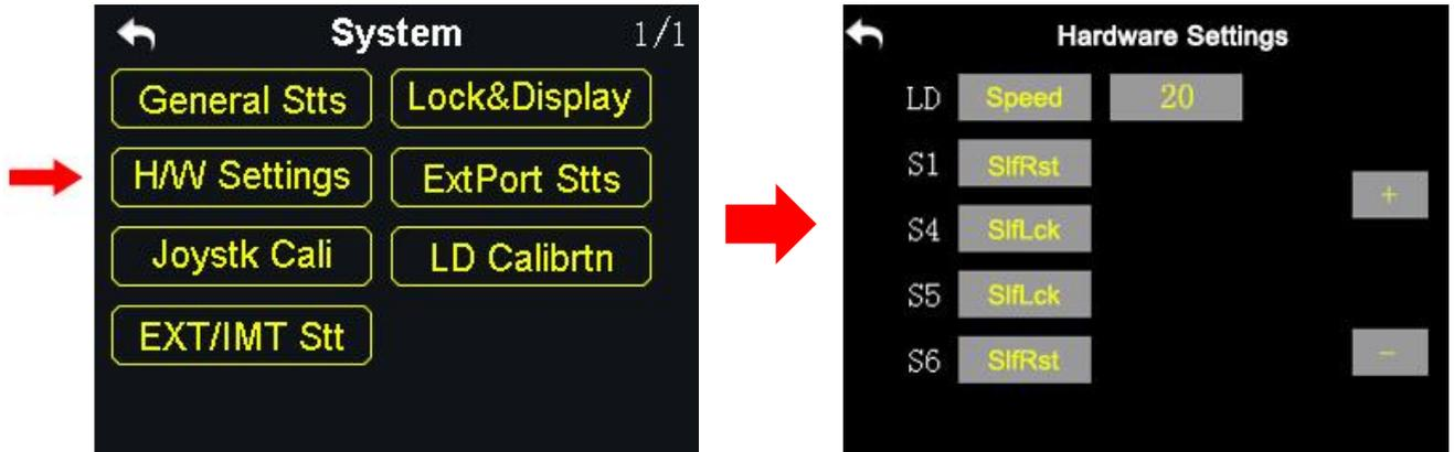
H / W settings help users do advanced settings for XT32 transmitter’s LD dial (switch between Position / Speed Mode) and S1 / S4 / S5 / S6 switches (switch between Self-locking / Self-resetting).
