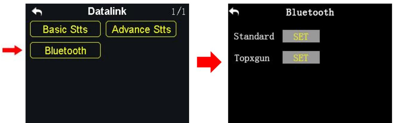
Before connecting transmitter to datalink ground station, please select the right external Bluetooth device according to your requiring flight controller.
