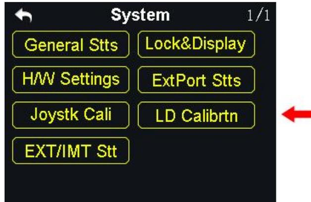
LD calibrating function helps users maintain LD dial's output accuracy. LD dial requires calibrating when it stays out of its middle position (channel output value is not 0) or fail to reach its maximum / minimum position.
