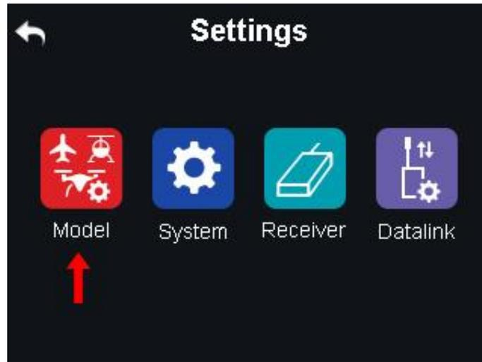
In XT32 transmitter's "Model Settings" menu there are a series of transmitter functions, offering basic and advanced settings for different kind of model devices.
