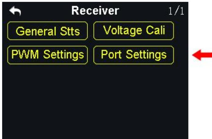
Port settings help users switch receiver DATA1/DATA2 port’s output mode (Receiver Extension / Data Telemetry) in transmitter
