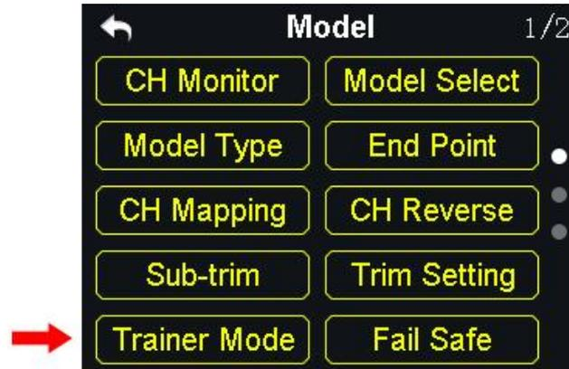
XT32 transmitter’s trainer mode helps experienced users train new talents. In trainer mode, two transmitters are connected with a trainer cable. Users decide which channel to do training.
