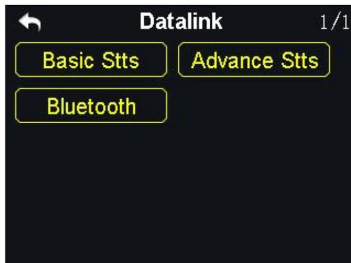
Basic Stts (Basic Settings): Set datalink module's basic functions.
