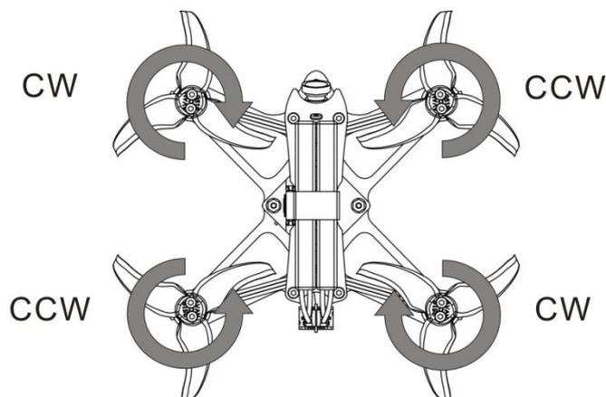
**Caution:** Failure to mount the propellers in the correct orientation will cause Tinyhawk Freestyle to not fly correctly and with no control. Please double check for the correct orientation.
