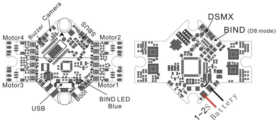
Tinyhawk Freestyle's main electronic board is shown above. This board contains a F4 flight controller with all 4 esc's and an 8CH/16CH receiver.
