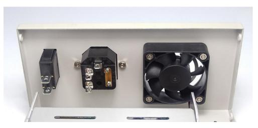
④Install the switch power supply: install the switch power supply on the lower board.
