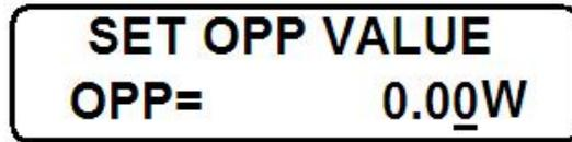
The default setting is 0, indicating that the OPP function is off. You can set non-zero data to start it, for example, set the maximum power of 20W, you can press the "< >" key to select the cursor position, and adjust the knob or press "↑", "↓" key to regulate the OPP value. After setting the output, when the actual output power exceeding 20W, the output will be cut off, then it will send an alarm and the screen will display error code E3.
