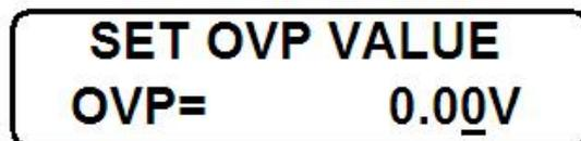
Users can move the position of cursor when pressing the “< >” key, rotate the adjust knob, regulate the voltage to 30.00V.
