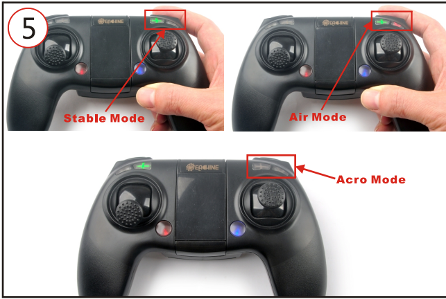
Press AUX2 switch(ch6) to select flight mode (Default is Acro mode)
