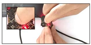
Another simple way to bind with the Flysky transmitter is: Plug the usb and go to the CLI command tab in the betaflight configurator, then type "bind\_rx\_spi", the receiver will getting into bind mode, and then make your Flysky transmitter to bind mode.
