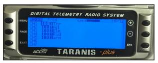
3. The default channel map for Cinecan Frsky version is TAER1234, please make sure your transmitter is matched, otherwise it will can't be armed. Toggle the AUX1 Switch , the Green LED on the flight controller will getting to be solid, this indicates the motor was armed. And also you can found "Armed" displayed on your FPV Goggles or the FPV Monitor. Please make sure keep the Cinecan level before arming. Be careful and enjoy your flight now!
