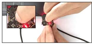
Another simple way to bind with the Frsky transmitter is: Plug the usb and go to the CLI command tab in the betaflight configurator, then type "bind\_rx\_spi", the receiver will getting into bind mode, and then make your Frsky transmitter to bind mode.
