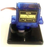
$\hfill\Box$  Use the two 7 mm screws to connect the two halves to clamp the servo
