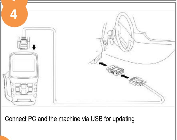
Connect PC and the machine via USB for updating
