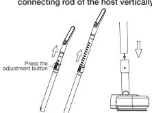
2 Place the host on the ground, push the active connecting rod on the host from horizontal to vertical. Connect the power cable in the metal tube.
