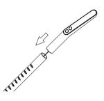
3 Press the adjustment button on the metal tube to stretch the tube to the longest, then insert it into the active connecting rod of the host vertically.
