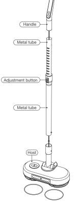
1 Press the latch on the metal tube to link the metal tube to the handle.
