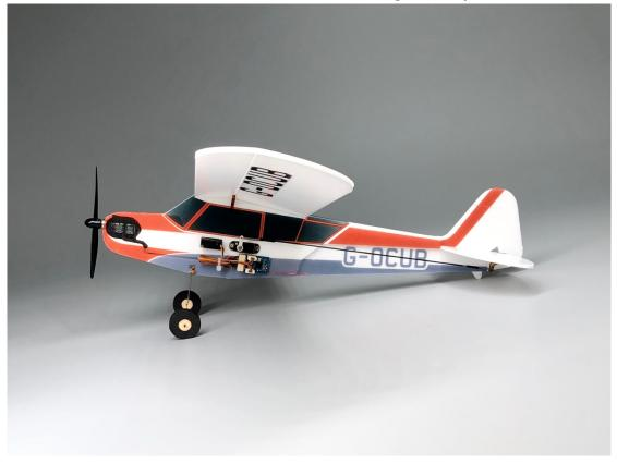
20. Attach the battery to the right side of the fuselage with nylon sticker.
