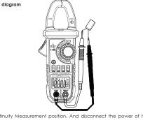
• Continuity Measurement 1, Set rotary switch to Continuity Measurement position. And disconnect the power of the circuit under test.
