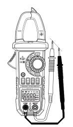
1. Set the rotary switch to proper Diode Measurement position, disconnect the p circuit under test, and press "SEL" key to select Diode Measurement function.  $2. \ \mbox{lnsert}$  the black probe into COM terminal and the red probe into INPUT terminal.
