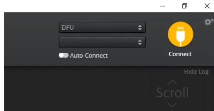
If you don't see DFU in the pulldown menu, then either the board didn't detect that you had the bootloader button pressed or your drivers are not installed correctly. If you don't see DFU in the pulldown menu, you cannot flash new firmware to the board. It won't work.
