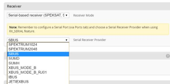
These are the most common serial receiver types that are likely to be encountered.
