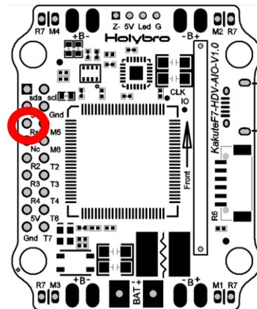
The GH port available on the board makes it much more convenient for you to connect HolyBro Kakute F7 HDV AIO to the DJI FPV VTx, for both signal and power supply.
