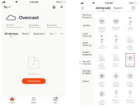
Turn on the battery switch, press the "RESET" button side of the base of the device and hold on for 5 seconds to enter into the Wi-Fi configuration state (the red indicator on the front flashes fast indicates that it is in the smart link configuration mode. If the indicator light flashes slowly, it indicates the AP configuration mode). The APP interface displays two modes which can be switched to each other before configuration start. As below:
