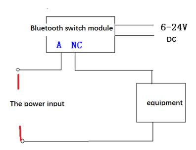
Simple speaking, relay module is to replace the traditional mechanical switch, as long as the mechanical switch can realize the function, can relay via bluetooth modules, if you don't know how to wiring, you can imagine if a mechanical switch for you, how to meet? This bluetooth
