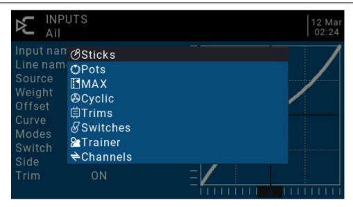
Weight: Normal range is a value between ± 100% will be zoomed to the gimbal operation. If you enter a negative value, for example -100% means reverse the output. Note that channel inversion should not use negative values on the Inputs page, and to reverse channels should be reversed on the Outputs page.
