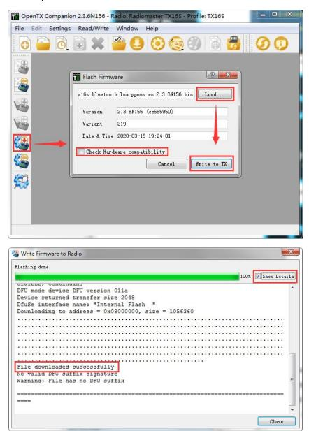
At this point, the firmware of the remote control is successfully written. Unplug the USB-C (TYPE-C) cable and you can use it after booting.
