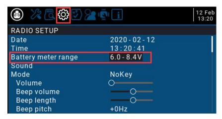
B. On the current page, turn the scroll wheel to find Battrey low (low voltage alarm), and fill in the alarm voltage as shown below. When the remote-control voltage is lower than the current set voltage, the system will play a voice and report that the battery voltage is low
