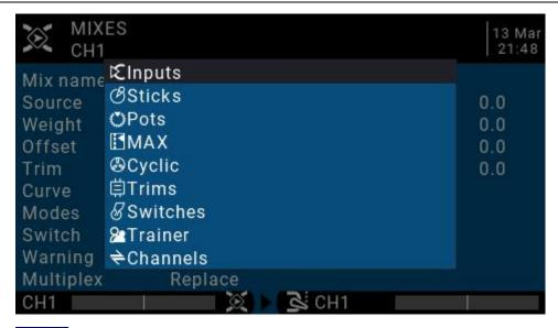
Weight: Channel travel amount, the range is -500 / + 500. The default value is 100. Negative values indicate reverse channel output.
