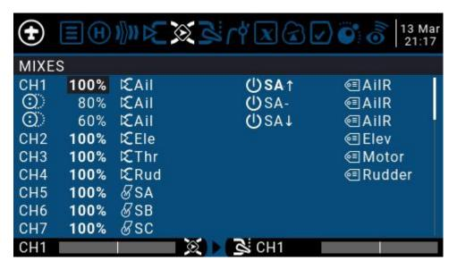
To edit a mixing control, use the scroll wheel to select the mixing control item up and down, and press and hold the ENT key to enter the editing submenu. Select Edit and press the ENT key momentarily.
