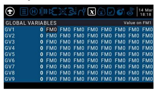
Modify the value directly or press and hold the ENT key to pop up the sub-menu to change the type and parameter of the global variable.
