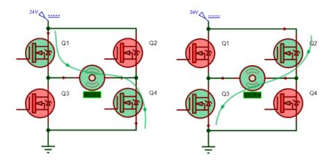
H-bridge is a popular motor control circuit. It is named because it looks like character "H" . It consists of four transistors/MOSFET, motor is connected on the center, you should through two transistors in diagonal line to drive motor.
