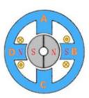
According to Ampère's circuital law, when current of coil A flow from left to right, stator generates magnetic field, internal side is North pole which will adopt rotator of motor. When the currents of four coils based on certain rule, they will generate a rotate magnetic field and drive the rotator rotate. If every motor has four rotators, it has four statuses:
