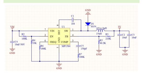
MP1584 regular supports wide 4.5V to 28V input, and up to 2A current output. Even thought that MP1584 support low to 4.5V input, however, VM also supply power for motor controller, which require at least 8.2V. So, the recommend input voltage is 8.2~28v.
