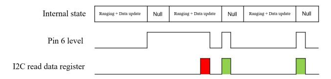
Figure 5 Timing of reading data register in I2C mode
