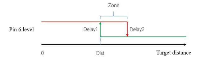
Figure 6 On/off mode that high level means closer
