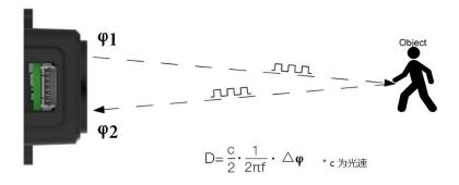
Figure 1: Schematics of TOF Principle
