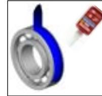
Apply a thin layer of threadlock on the external part of the ball bearing
