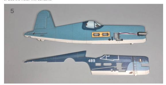
6. Glue both sides of fuselage together.
