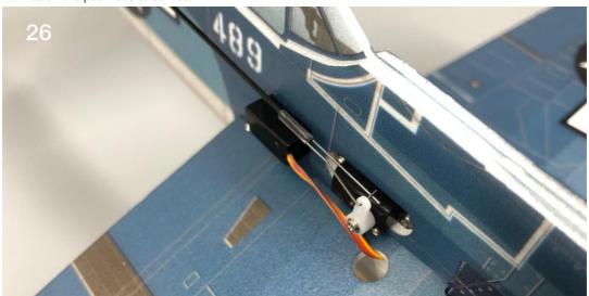
27. Attach the pushrods to control horns.
