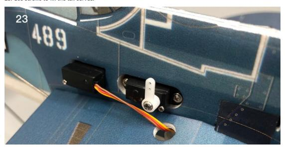
24. Glue the elevator & rudder control horns.
