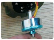
3. Tighten the engine. (The assembly steps of the left side is the same as the last step.)
