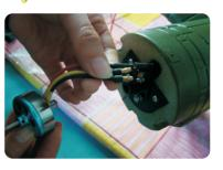
2.Insert the engine into the correct position of the base.
