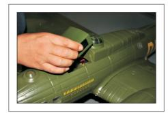
Put the battery into the cabin first, and the connect the power line.
