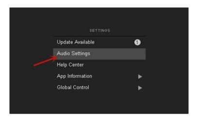
② Select active input channels. If XTONE(Duo)'s INL input is connected, select XTONE1; if XTONE(Duo)'s INR input is connected, select XTONE2. Then adjust the Audio Buffer Size to 64 samples and activate XTONE as MIDI Inputs.
