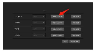
(3) Click "MIDI Learn" at TOGGLE to start MIDI specification. the "Waiting for MIDI CC" appears on the screen. Press the foot switch on XTONE(Duo) that you want to use to toggle this pedal. Then MIDI function is successfully specified.
