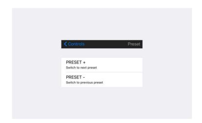
(3) Click MIDI Learn, the "Waiting for MIDI CC" appears on the screen. Press the foot switch on XTONE(Duo) that you want to use to switch presets. Then MIDI function is successfully specified. Go back to the main page and you can press the foot switch to switch presets.
