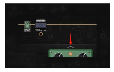
② Long press the indicator position of the pedal to open the MIDI specification.
