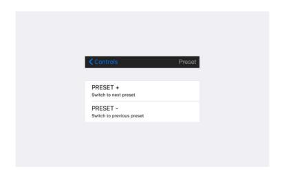
(3) Click MIDI Learn, the "Waiting for MIDI CC" appears on the screen. Press the foot switch on XTONE Pro that you want to use to switch presets. Then MIDI function is successfully specified. Go back to the main page and you can press the foot switch to switch presets.
