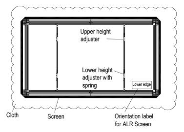
4.4 Attach the screen onto the inner frame using the tension springs. Install the tension springs to the four corners in the sequence 1~8 first. Then install the other tension springs to both sides from the frame center as shown below (please pull the springs with force at the same time).
