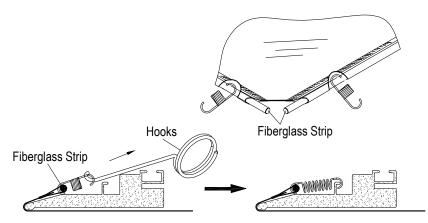
4.5 Place the screen upright to check its evenness. Adjust the spring until no wrinkles observed.
