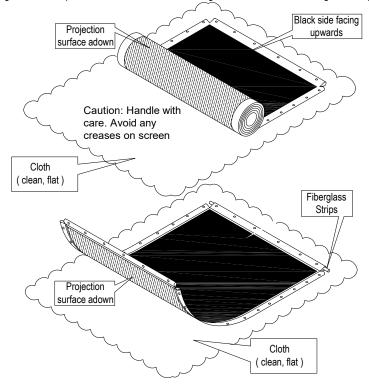
4.3 Put the installed inner frame onto the back side of the screen. Put the installed frame onto the screen. Pay attention to the labels on the screen for the right orientation and align them well by referring to the marks on the four corners of the screen.
