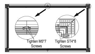
$3.5\,$  Fix the two struts onto the sliders with the included M5\*7 screws. Keep them paralleled with each other with a distance of  $110\,\text{cm}$  /  $43.3\,\text{in}$ .
