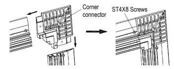
3.4 Assemble the inner horizontal frames with the vertical ones.
