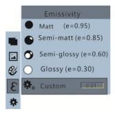
As shown in the figure, press "key to enter the main menu and select "(emissivity) option and press "button to enter the emissivity list.
