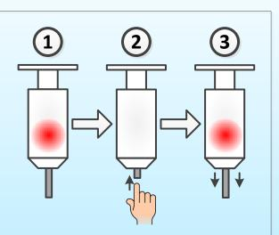
Send that command and use your finger to retract the pin. The sensor should trigger (2). It must come back to its « probing » position at end (3).
