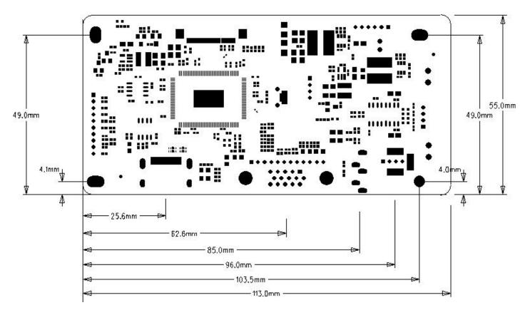
Remarks: PCB thickness + height of the highest part≤14.5mm
