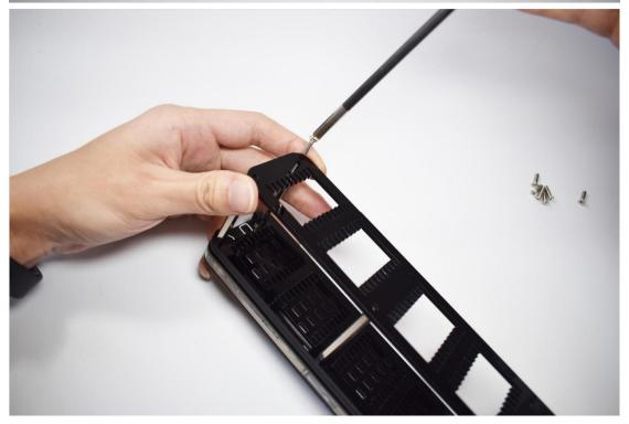
32.Install screws at two diagonal corners
