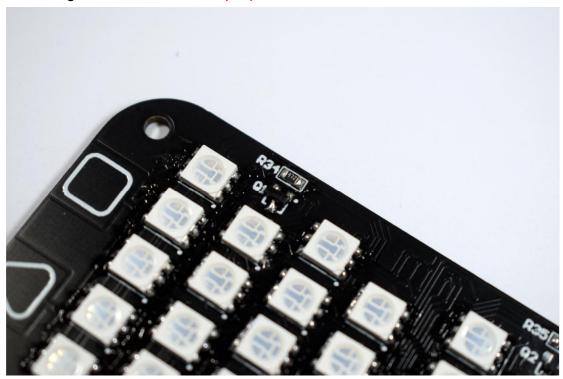
6. The LED, resistor and transistor are welded as shown below
