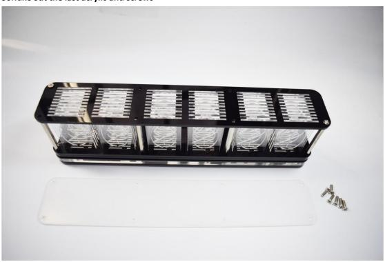
37. When installing this acrylic board, pay special attention to that, when installing the transparent acrylic, you must first install a screw to press it, and then remove the screws that pressed the black acrylic before re-fixing it.
