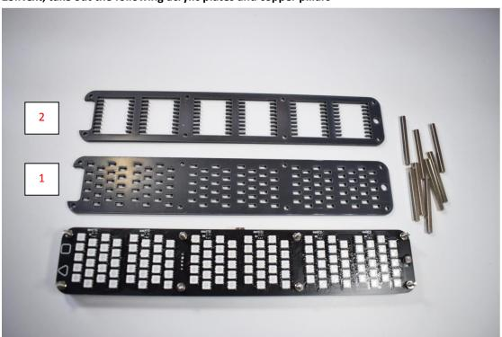
24.Tear off the protective film, and install this acrylic board on the circuit board. Please note that the holes here should correspond one by one, don't install it backwards, the LED will not show light if it is installed backwards
