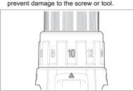
The torque specifications shown here are approximate values obtained with a fully charged battery pack
