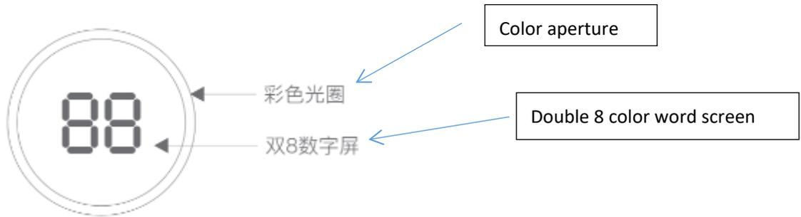
The display has a three-color aperture (red, blue, purple). After the machine is turned on, the aperture starts to light up. When the ambient humidity is **above 70**, it displays **red**; when the ambient temperature is **below 50**, it displays **purple**, and when the ambient humidity is **50-70** **Blue** is displayed between.
