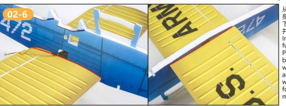
从02-4切开的口插入下机翼到机 身,注意机翼正反,有字一面朝 下, 调整机翼居中后, 按压粘固 并随预留槽使机翼呈一定弧度。 Insert the lower wing into the fuselage from the cut in 02-4. Pay attention to the front and back of the wing, with the words facing down. After adjusting the center of the wing, press and fix it and follow the reserved groove to make the wing curve.
