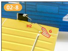
翼上。 After adjusting the servo horn, spread the foam glue to fix the servo horn on the aileron.
