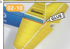
把水平尾翼插入机身 尾部,连接处用泡沫 胶粘固。 Insert the horizontal tail into the tail of the fuselage, and fix the joint with foam glue.
