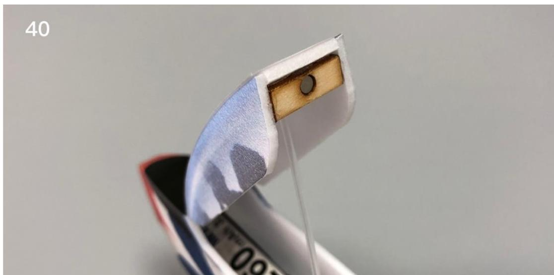
Install magnet base on the fuselage.
