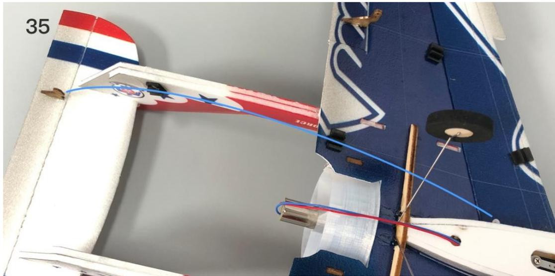
Use 502 glue to fix an 80mm duct on the base.
