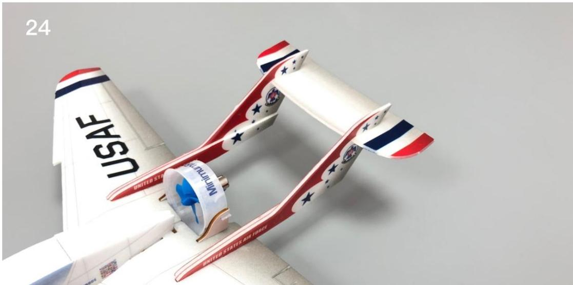
Paste the sticker on the top of the fuselage to form a hinge connection for the hatch cover to be turned over. Glue can be used at the hinge joint to increase strength.
