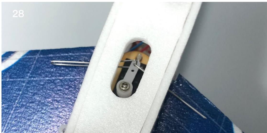
Fix the aileron duct seat with glue. The distance between the two seats and the fuselage and aileron control horn are 30mm.
