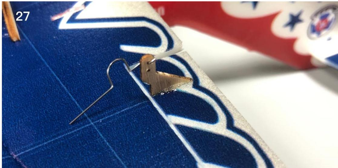
Attach the pushrod clip on the same hole of aileron servo arm.
